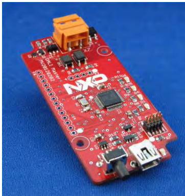
Fig 1. OM13046 USB to DALI Master assembled PCB
